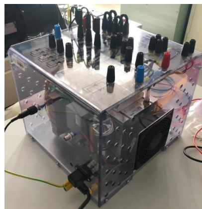
Figure 3 : SEMITEACH Thyristor Power Electronics Teaching System [4].
